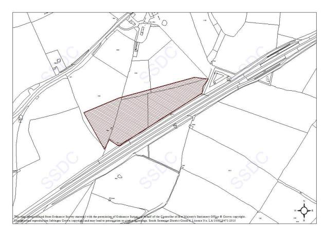
This application is seeking alterations to an approved scheme for an acoustic barrier (planning consent 10/02210/FUL). The alterations include raising the bund height by up to approximately 2 metres above that approved as well as the slight remodelling of its form. It is understood that these revisions are sought as the approved bund, which is still under construction, does not appear to be as effective in reducing traffic noise from the A303 to the landowner's property Riding Gate Cottage.
